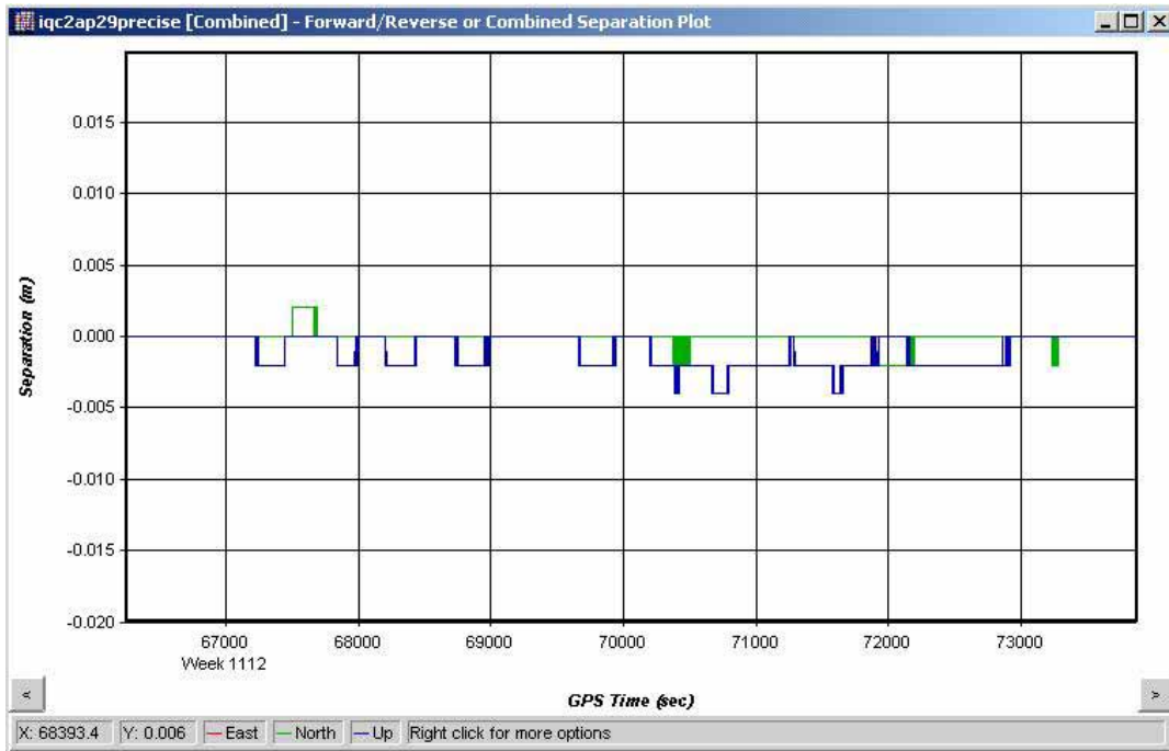
Figure 5: Coordinate difference when using precise ephemeris
