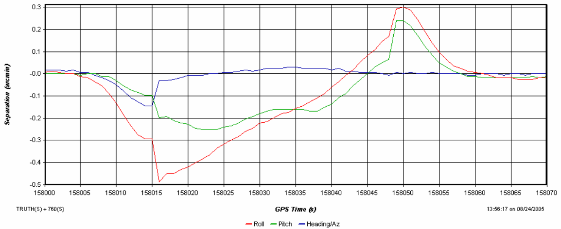
Figure 31: Attitude error in combined RTS processing during 30 second GPS outage
