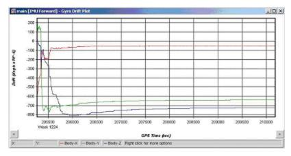
Figure 5.27 IMU Gyro Drift Plot
