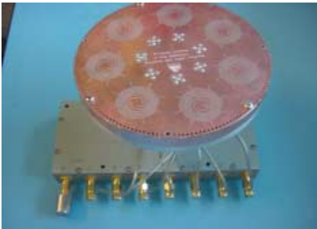
Figure 1. 7-element CRPA array with 8-way combiner
