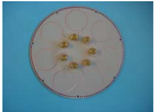
Figure 2. 7-element CRPA array (bottom side)
