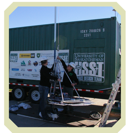
Figure 3: Members of the USST team attach the climber to the ribbon
