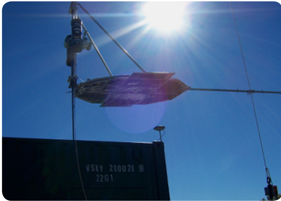
Figure 1: A NovAtel GPS-702-GG antenna guides the USST's elevator cab up the ribbon at the 2007 X-Prize Cup
