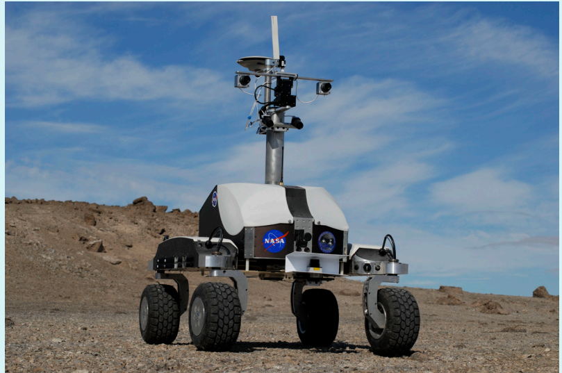
Figure 1: K-10 Black rover uses its ground-penetrating radar in a polar desert Photo Credit: NASA Ames Research Center
