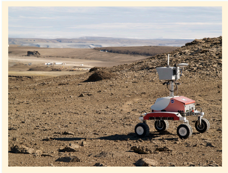
Figure 4: K-10 Red rover uses its 3-D scanning systems during field tests in the "frost rubble zone" of Earth Photo Credit: NASA Ames Research Center
