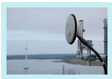
Figure 6: External NovAtel Antenna Onboard Ship Photo Credit: S. Martin, Astrium GmbH, Munich, Germany, 2007
