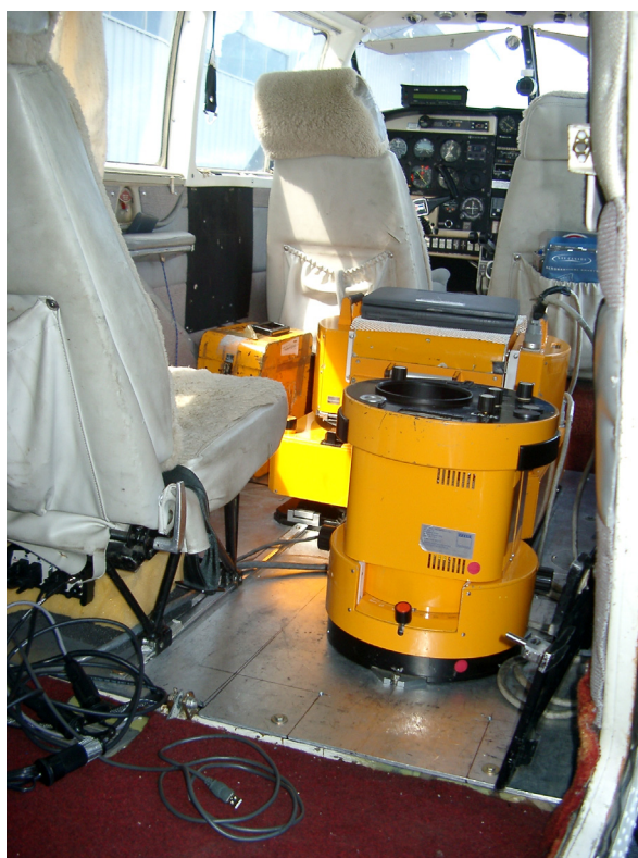
Figure 5. LMK Camera System Mounted in Aircraft
