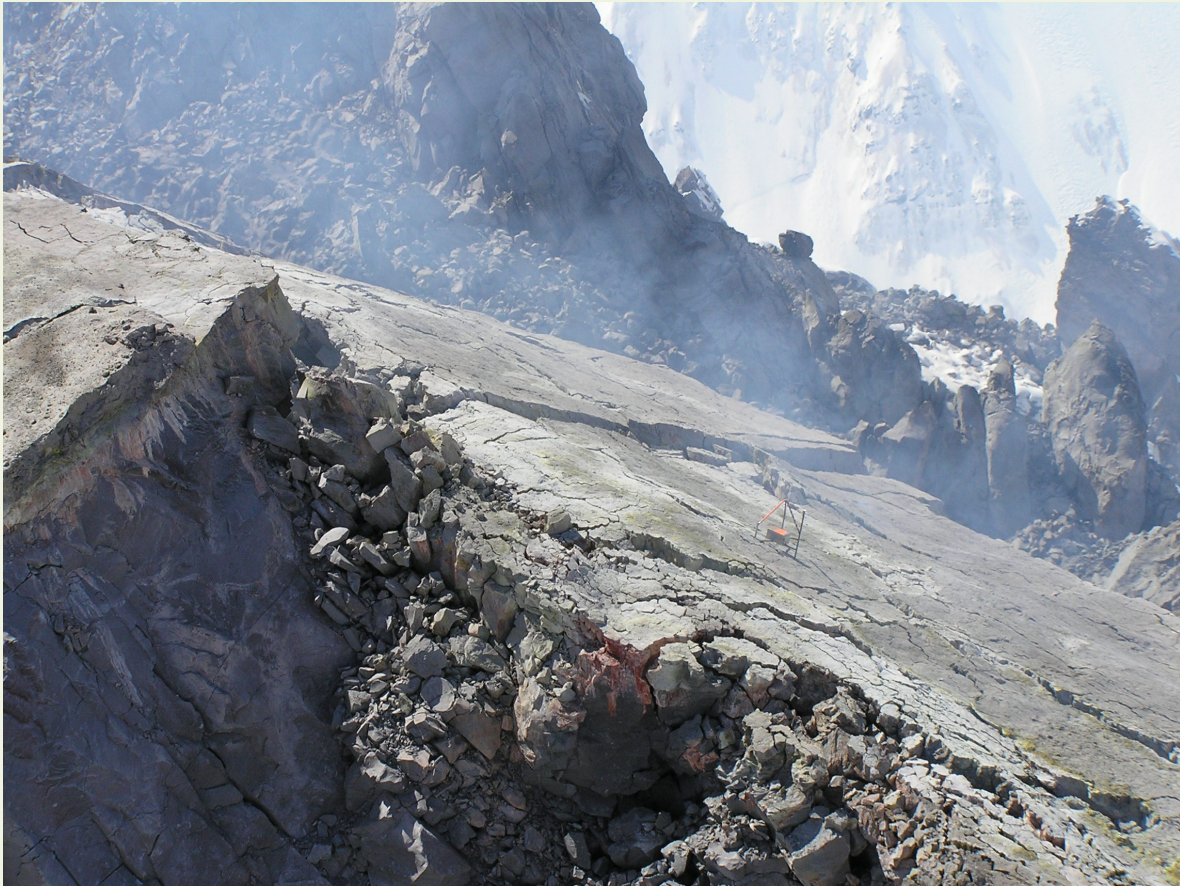
Figure 1: Spider measuring the rate of the lava dome extrusion using a NovAtel receiver at Crater, Mount St. Helens, Washington
