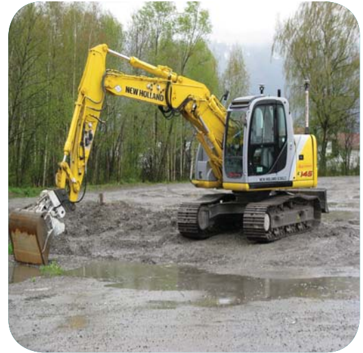
Figure 2: One antenna is the master and one antenna is the remote on this digger. They receive corrections from an external RTK base (not shown).
