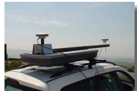
Figure 4: Antenna setup in a dynamic van test
