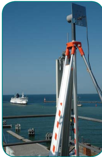
Figure 1: A static base antenna with one or more rover ships in port.
