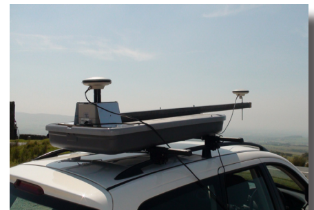
Figure 4: Antenna setup in a dynamic van test
