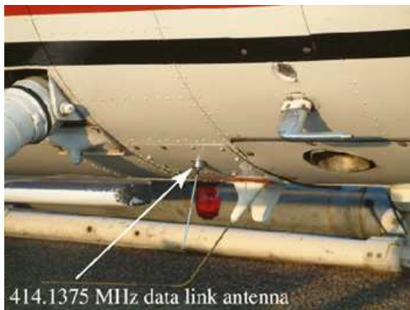
Figure 11. BO-105 RF data link antenna installation, left side of airframe.
