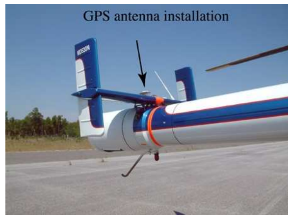
Figure 14. L1/L2 GPS antenna installation on the MD520N.
