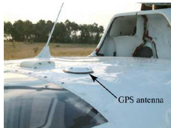
Figure 8. BO-105 GPS Antenna Detail.
