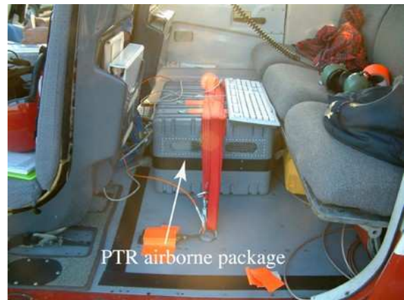
Figure 13. PTR airborne package installation in the BO-105.
