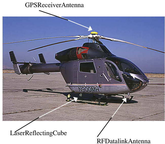
Figure 2. MD900 Explorer With Antenna Installations.
