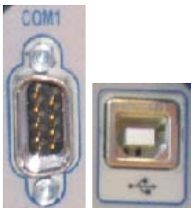
Figure 4: COM1 Port (left) and USB Port (right)
