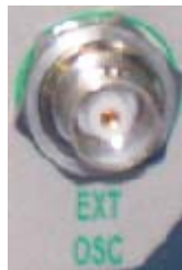
Figure 14: External Oscillator Port
