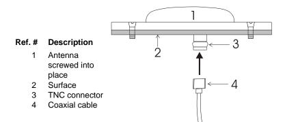
Attach the other end of the coaxial cable to the antenna input port of the receiving device, which must provide power as detailed in the SPECIFICATIONS section of this guide. All NovAtel GPS receivers provide the necessary power through their antenna RF connectors.
