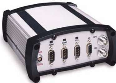
Figure 4: Receiver Enclosure Back Panel
