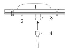
6. Attach the other end of the coaxial cable to the antenna input port of the receiving device, which must provide power as detailed in the *SPECIFICATIONS* section of this guide. All NovAtel GPS receivers provide the necessary power through their antenna RF connectors.
