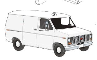
The graphic above shows examples of where the 534 antenna may be placed on an aircraft or vehicle (not to scale).
