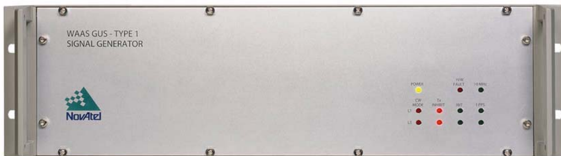
Figure 1: Galileo Test Signal Generator
