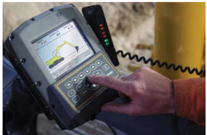
Top: The Trimble GCS900 uses dual GPS receivers and solid-state sensors to measure the 3-D position of the bucket tip. Bottom: The CB430 operator control box provides visual guidance to the excavator operator.
