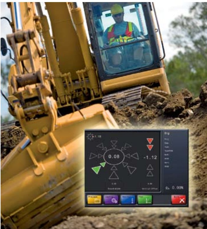
Leica's DigSmart 3D system includes a graphic color monitor in the cab that displays project design information and 3-D GPS position.
