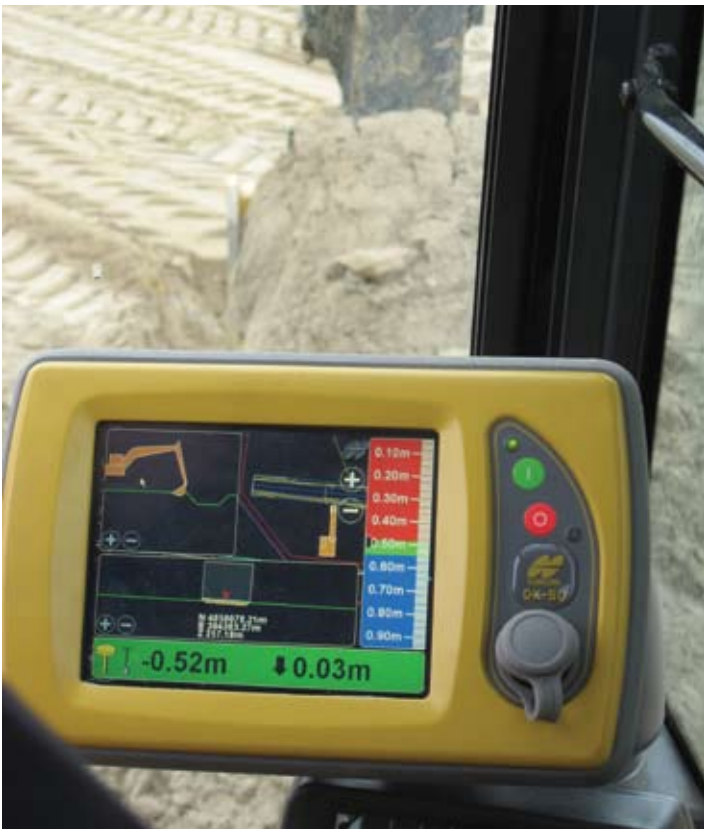
Shown is the Topcon GX60 control box with touch-screen display running 3D-MC software. The display is “split” in multiview so the operator can monitor plan view, profile view, cross section, as well as the Virtual Grade Rod.
