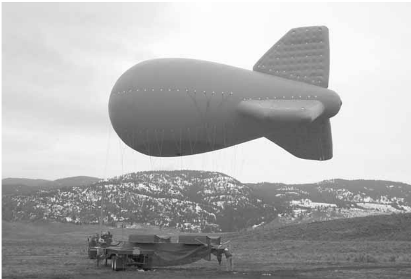
▲ AEROSTAT prototype, 1/3 scale, at launch for its first flight in Pentiction, British Columbia, Canada in March 2002
