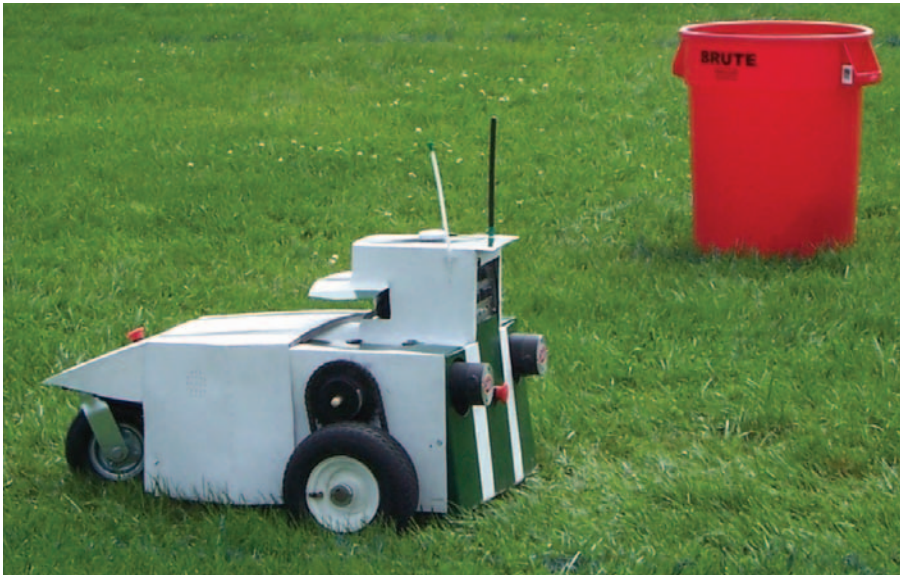
▲ THE OHIO UNIVERSITY autonomous lawn mower navigates past an orange barrel obstacle on its first pass at a marked cutting plot. OU students upgraded the university's mower from last year's competition to sport chain drives and more-powerful DC drive motors (evidenced by two red safety switches). Antennas help deliver GPS, WiFi differential GPS, and remote shut-off capabilities.
