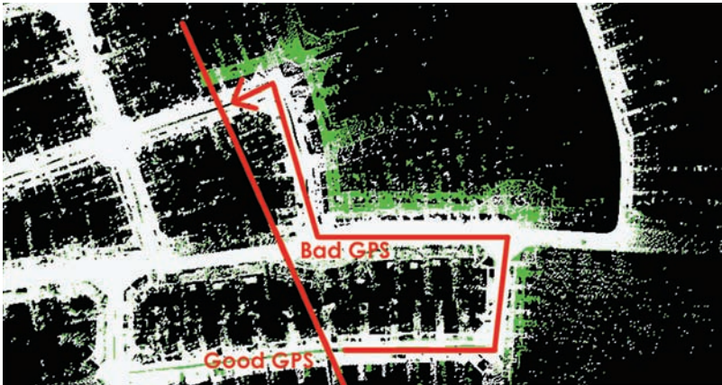
▲ FIGURE 5 depicts the processed point-clouds associated with a post-Afghanistan urban project where numerous cycle slips occurred. In the absence of GPS, the GPS/IMU solution drifts with time as shown by the green point cloud. Further optimization of the processing algorithms and methodologies allows for full recovery of drift-free trajectories, as depicted by the white point cloud.
